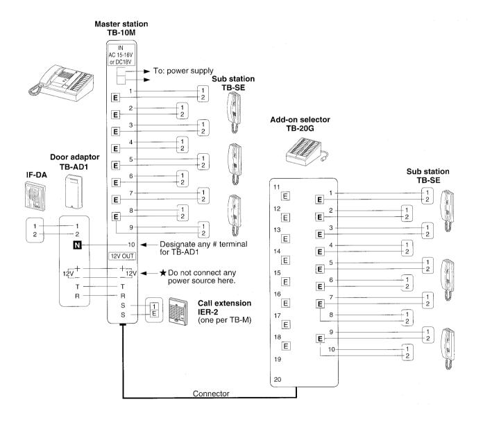
★ Up to 3 TB-AD1 door station adaptors per TB-M. 5 wires homerun to TB-M.
